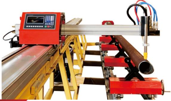
Portable CNC plate/pipe cutting machine can achieve two kinds of pipe and plate cutting method, can greatly save customers cost. The guide rail for the round pipe support is 24kg/m fine grinding rail, it has heavy bearing capacity, long life and other advantages. Chuck axis use high precision gear and servo motor drive, low noise, high precision, long service life. Adjustable screw for pipe support frame is using precision T-screw, when support the workpiece can adjust smoothly.
