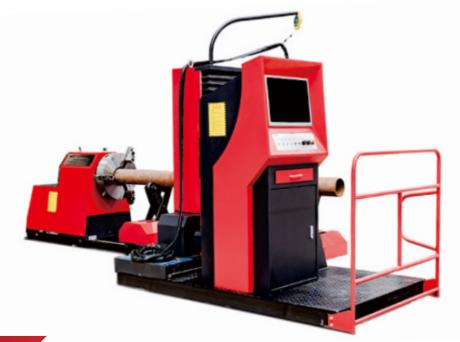
MS-6XG Intersection cutting machine has 6-axis, it can custom 8-axis. This machine can cut different diameter of intersecting line hole, meet the vertical axis and axis condition branch director and no eccentric. The machine can also cut cylinder intersection line at the end of branch pipe, meet the pipe axis and the eccentric and no eccentric director axis intersecting condition.
