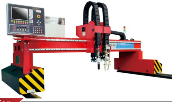
B-series heavy gantry plasma flame cutting machine uses plate tenon and mortise welding gantry, with bilateral servo drive. The end beam uses an externally mounted roller structure, which is stable in movement and easy to adjust. It can achieve high-precision cutting with high-precision reducer and rack. The machine uses industrial CNC system, such as Hypertherm, Beckhoff, Fangling. It is an ideal model for large and medium-sized enterprises to cut steel plates with high accuracy and stability.
